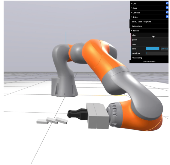
Fig. 11: Dominoes Knocked Over: Robot knocks over dominoes, showing the correct spacing between them.
